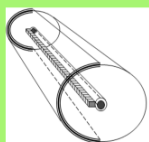
Fig. 2 Proposed arrangement of hybrid PV + TE solar converters
